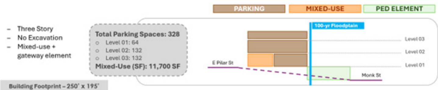
Figure 2.6. Parking Facility Proposed Cross Section
